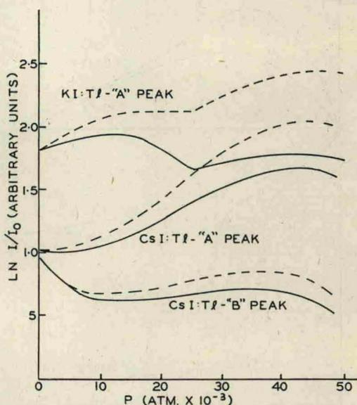
FIG. 6. Variation of peak intensity with pressure.
