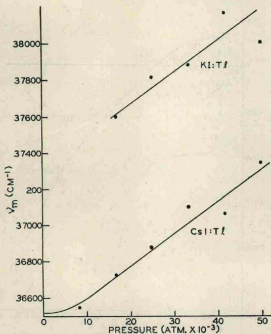
FIG. 5. 'B' peak frequency shift versus pressure.
